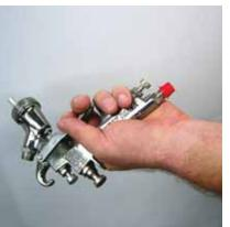
This is especially necessary when using waterborne solvents. The spray gun needs to be dried off completely **inside and out** to eliminate any cleaning solution remnants on the gun surface or inside the gun. All of our guns fluid passages are stainless steel, but if cleaning solution makes its way inside the spray gun air passages and remains wet, it can cause corrosion on the raw aluminum gun body. After drying **inside and out**, make sure all moving parts and packings are lubricated.
