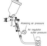
The gun should be held so that it is perpendicular to the surface of the work piece at all times. Then, the gun should move in a straight and horizontal line. Arcing the gun causes uneven painting.
