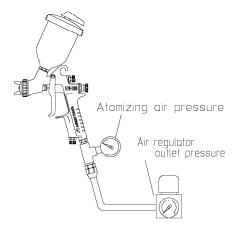
Pulling the trigger of the gun with the pattern adj. set and air adj. set fully opened adjust the air regulator in the spray booth to obtain 1.0~1.3 bar (14~18 PSI) at the gun inlet as issued on specifications table ahead. In this way the gun will atomize within 0.7 bar (10 PSI) inside air cap.
