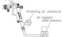
The gun should be held so that it is perpendicular to the surface of the work piece at all times. Then, the gun should move in a straight and horizontal line. Arcing the gun causes uneven painting.
