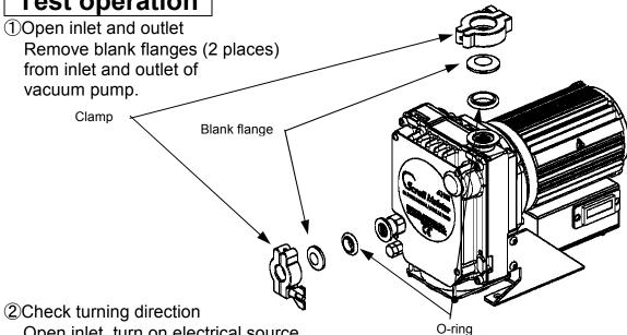
Open inlet, turn on electrical source to start operating vacuum pump and check that comes out of air outlet.
