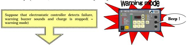
Job - 1 Suspend coating job and check failure item by lit-up position of failure display lamp.
