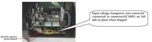
Job - 2 Change input changeover wire connector on electric source print board fitted to back lid to 200V setting position.
