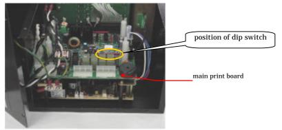
Job - 3 Change dip switch(No.2) on removed electric source print board from ON to OFF.
