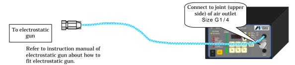
**4.3** Connection of external charge signal wire (only auto gun type[E-A10 series])
