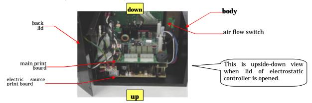
Job - 3 After setting print board, close controller body and back lid, and fix with screws.
