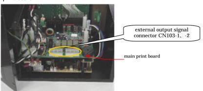
Job - 3 Connect external output signal wire to charge input signal wire terminal block on main print board.
