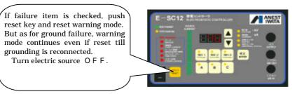
Job - 3 After cancelling warning mode, proceed confirmation about checked failure items according to below chart. When failure is still detected, equipment may have failed. Check again 8 Problems and remedies J.
