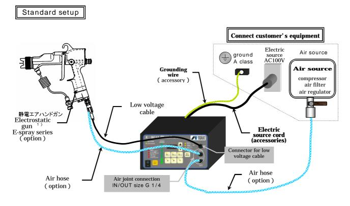
1 )In case of auto gun type, you do not need to connect electrostatic controller to air hose. But 4.3 connection of external charge signal becomes necessary.
