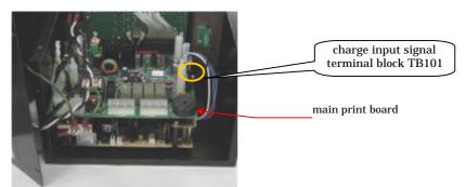
Job - 3 Connect external charge signal wire to charge input signal wire terminal block on main print board.
