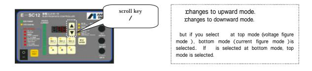
Job - 2 Lamp lights up in selected display mode and present figure of selected mode is displayed on 7 seg. display lamp.
