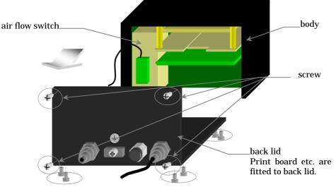
Job - 2 Electric source print board and main print board are fitted to electrostatic controller.
