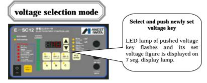
Job - 3 If fixed key is pushed, voltage set mode returns to normal mode. Charge from next time is set figure by newly selected voltage key.
