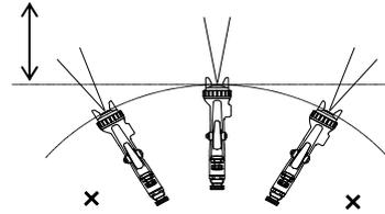
Pulling the trigger of the gun with the pattern adj. Set and fully opened adjust the air regulator in the spray booth to obtain 1.0~1.3 bar ( 14~18 PSI) at the gun inlet as issued on specifications table ahead. In this way the gun will atomize within 0.7 bar (10 PSI) inside air cap.
